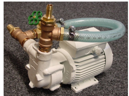
Pump C 80 with bypass and manually flow restriction
