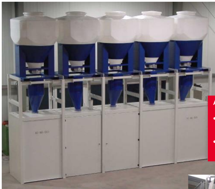
FD 5 DS with special equipment PVC-silos 1,2 m³
