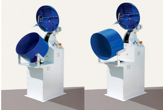
EasyMix 30/50 K discharging of the mixing pan (motor-driven)
